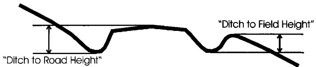
Figure 24 Road cross-section Ditch-to-Field and Ditch-to-Road heights
