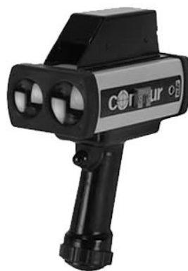
Figure 5.4. A typical hand-held distance meter (photo: LaserCraft Inc., 2007).
