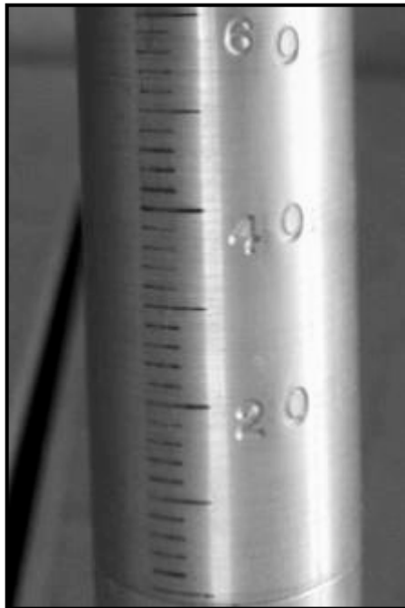
Figure 4.10. Detail of Standard Federal spring scale. Units are in 2 cm intervals of SWE, while the interval between tic marks is 2 mm.
