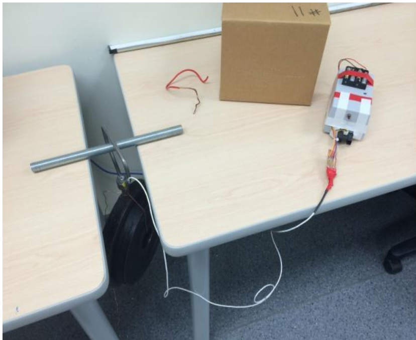
Figure 9: An example of calibrating tension sensor values
