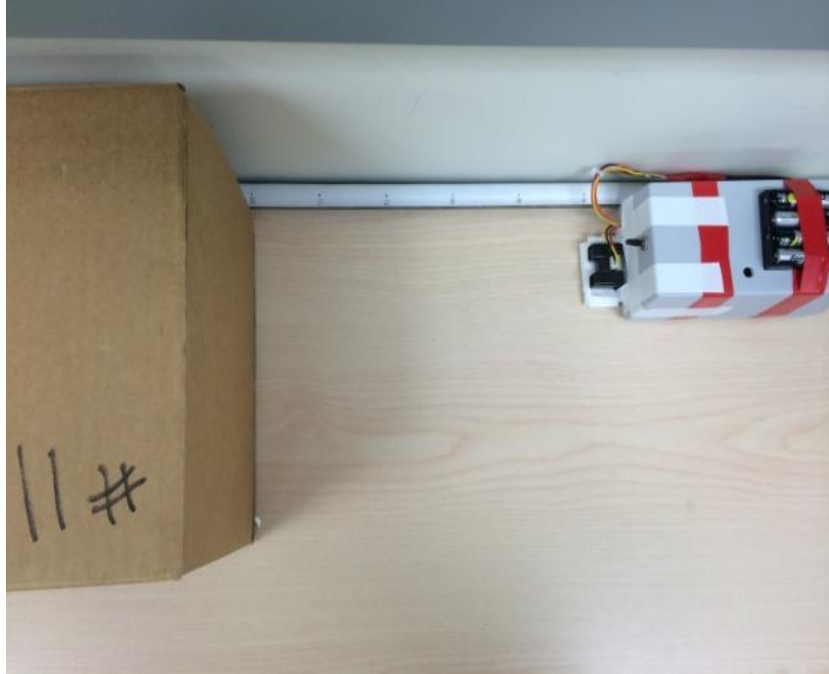
Figure 8: An example of calibrating distance sensor values
