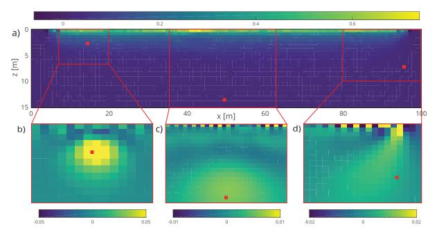
Figure 5.3 – a) Diagonal of the resolution matrix reshaped into a 2D grid. b)-d) Rows of the resolution matrix (point-spread functions) corresponding to the locations denoted by the red dots in the zoomed sub-figures. Note that different color scales are used in each panel in order to highlight the characteristic features.
