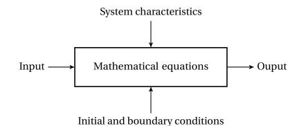
Figure 1.2 – General structure of the mathematical model in link with model design. Adapted from Essink (2000, p. 9)
