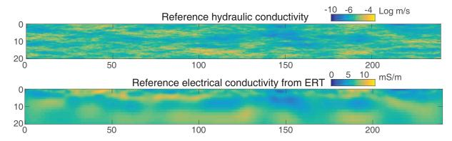
Figure 4.4 – (Top) Reference hydraulic conductivity field; (bottom) low-resolution electrical conductivity structure estimated from surface-based ERT.
