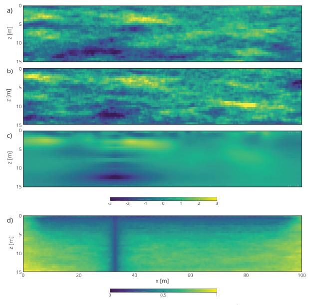
Figure 5.7 – Results of stochastic simulations. a) True initial field  $\mathbf{z}^{true}$ , b) example of a realization  $\mathbf{z}_c^{sim}$ , c) mean of 500 realizations  $\overline{\mathbf{z}_c^{sim}}$ , and d) standard deviation of the same 500 realizations std ( $\mathbf{z}_c^{sim}$ ).
