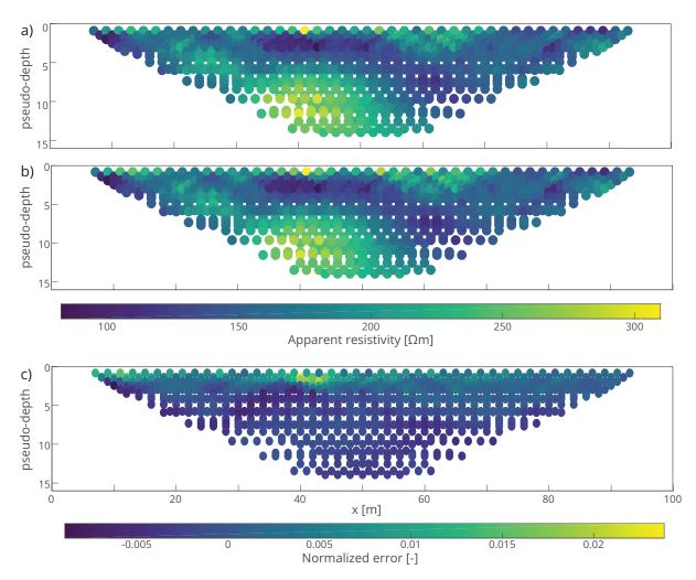
Figure 5.10 – Comparison of the pseudo-sections of the apparent resistivity. a) Observed apparent resistivity and b) the mean forward response of 500 stochastic realizations, and c) the normalized relative error of the realizations  $(f(\boldsymbol{\sigma}_{c}^{sim}) - \mathbf{r}^{obs})/\mathbf{r}^{obs}$ .
