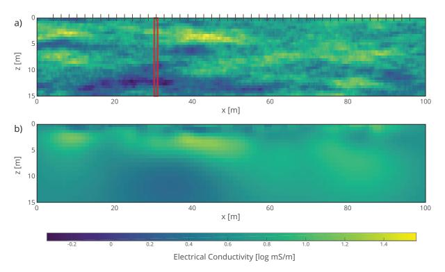
Figure 5.1 - (a) True fine-scale electrical conductivity field and (b) corresponding surfacebased ERT estimate. The red rectangle denotes the location of a borehole, along which the true electrical conductivity is known. The brown vertical line segments in (a) indicate the locations of the 47 electrodes used.
