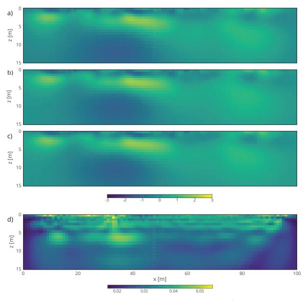
Figure 5.9 – Results of the stochastic simulations. a) Inverted field  $Z^{est}$ , b) upscaled version or G-transform of a single example of realizations  $RUz_c^{sim}$ , c) mean of the G-transforms of 500 realizations  $\overline{RUz_c^{sim}}$ , and d) standard deviation of the G-transforms of 500 realizations std  $(RUz_c^{sim})$ .
