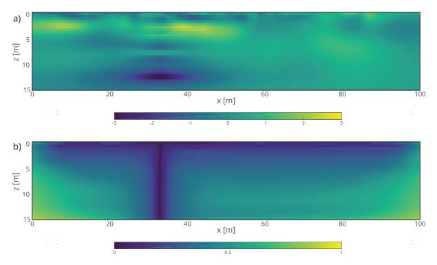
Figure 5.6 – a) Co-kriging estimation based on the tomographic image and the hard data  $\hat{z} = \Lambda_z z^{hd} + \Lambda_Z Z$  and b) corresponding co-kriging error variance.
