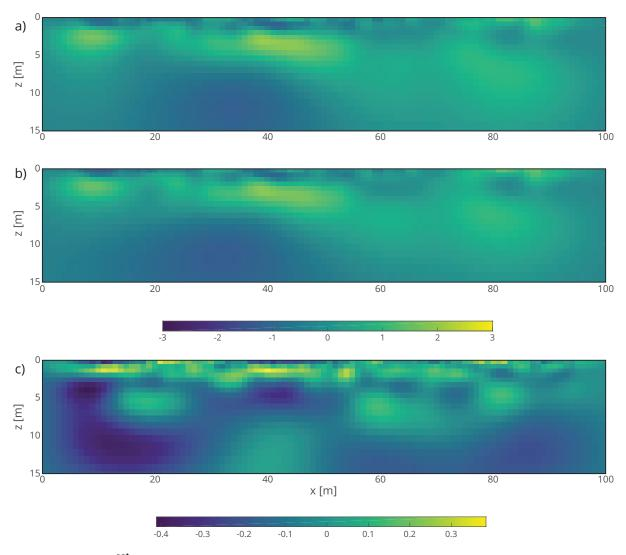
Figure 5.4 – a)  $\mathbf{Z}^{\text{est}}$  resulting from the tomographic inversion, b) G-transform of the true field  $\mathbf{G}\mathbf{z}^{\text{true}} = \mathbf{R}\mathbf{U}\mathbf{z}^{\text{true}}$ , and c) difference between the two.
