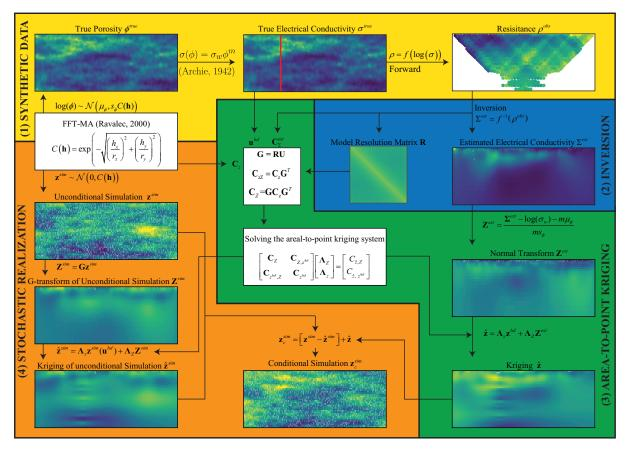
Figure 5.2 – Schematic overview of the key elements of the proposed methodology involving (1) generation of synthetic data (yellow), (2) geophysical inversion (blue), (3) area-to-point kriging (green), and (4) conditional stochastic simulation (orange).
