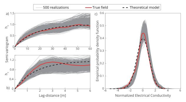
Figure 5.8 – Horizontal and b) vertical semi-variograms, and c) probability density function based on 500 realizations (grey lines) with the values for true field (red line) and the theoretical model (dashed black line) superimposed.
