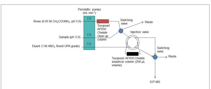
FIGURE 1 | The FI manifold with on-line preconcentration and ICP-MS detection for the determination of iron in seawater. Reprinted from Clough et al. (2015). Uncertainty contributions to the measurement of dissolved Co, Fe, Pb, and V in seawater using flow injection with solid phase preconcentration and detection by collision cell – quadrupole ICP-MS, Copyright 2015, with permission from Elsevier (Clough et al., 2015).
