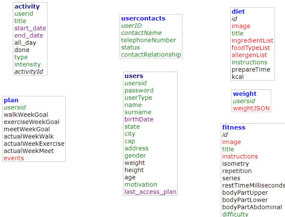
Figure 22 - remote_assistan database schema
