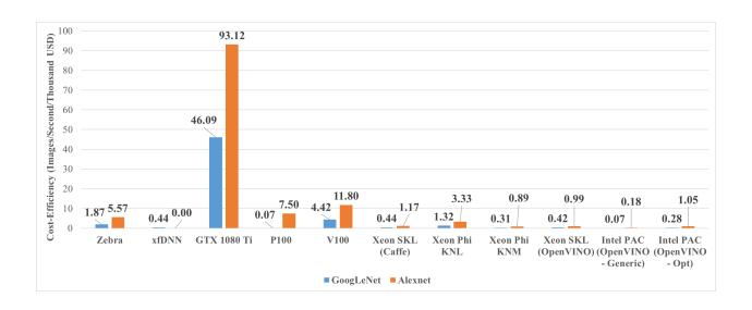
Figure 18 Cost-Efficiency Characteristics of CNNs Across All Devices and Frameworks
