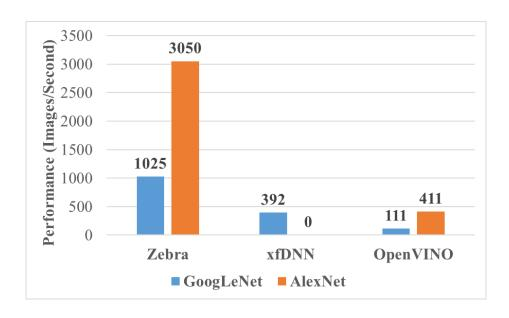
Figure 12 Performance of Caffe-based Frameworks on Xilinx FPGA and OpenVINO on Intel PAC FPGA
