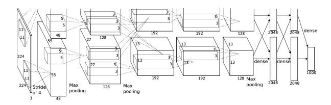
Figure 1 Dual Data-path Design of AlexNet [17]
