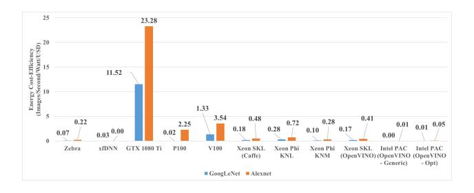
Figure 19 Energy Cost-Efficiency Characteristics of CNNs Across All Devices and Frameworks
