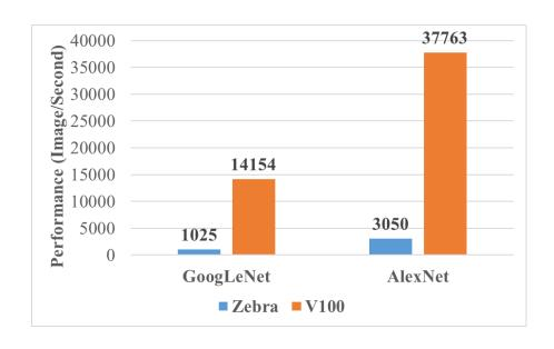
Figure 14 CNN Performance on Xilinx FPGA Using Zebra and Tesla V100 GPU
