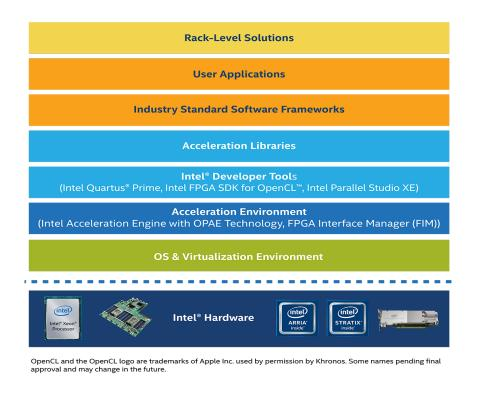
Figure 2 Intel Acceleration Stack Featuring OPAE [33]
