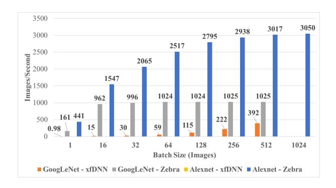
Figure 6 CNN Performance Across Xilinx FPGA Frameworks with Varied Batch Sizes
