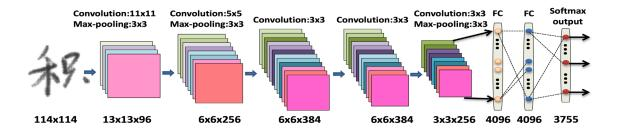
Figure 4 Architectural Design of HCCR-AlexNet [11] Referred to as Alexnet in This Research
