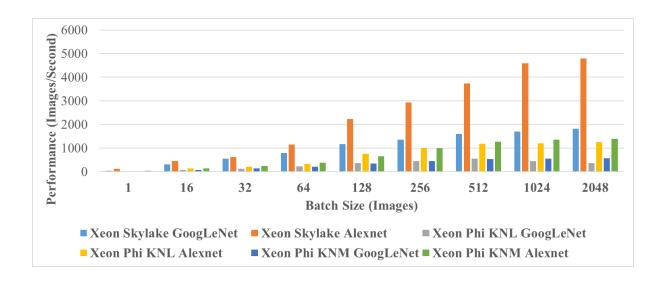
**Figure 9** CNN Performance Across CPU Devices using Hyper-threading with Varied Batch Sizes (See Appendix for Values)
