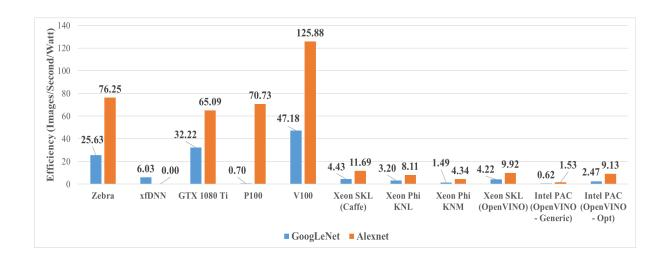
Figure 17 Efficiency Characteristics of CNNs Across All Devices and Frameworks
