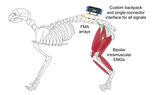
**Figure 5.** Summary of implanted hardware. This cartoon displays the floating microelectrode arrays (FMAs) and their gold wire bundles in the spinal column as well as the muscles targeted by intramuscular electromyography (EMG) electrodes and their leads in green. These wires were routed percutaneously to the custom backpack, which was mounted to the fascia above the dorsal laminectomy.
