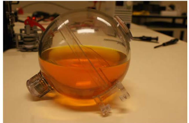
Fig. 5 Tank half filled with Novec liquid on earth
