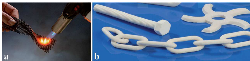
Fig. 3 Examples of ceramic parts manufactured by stereolithography. a SiC ceramic mesh manufactured by HRL (Courtesy of HRL Laboratories, Photo by Dan Little) [40] b Alumina parts (Courtesy of CTTC)
