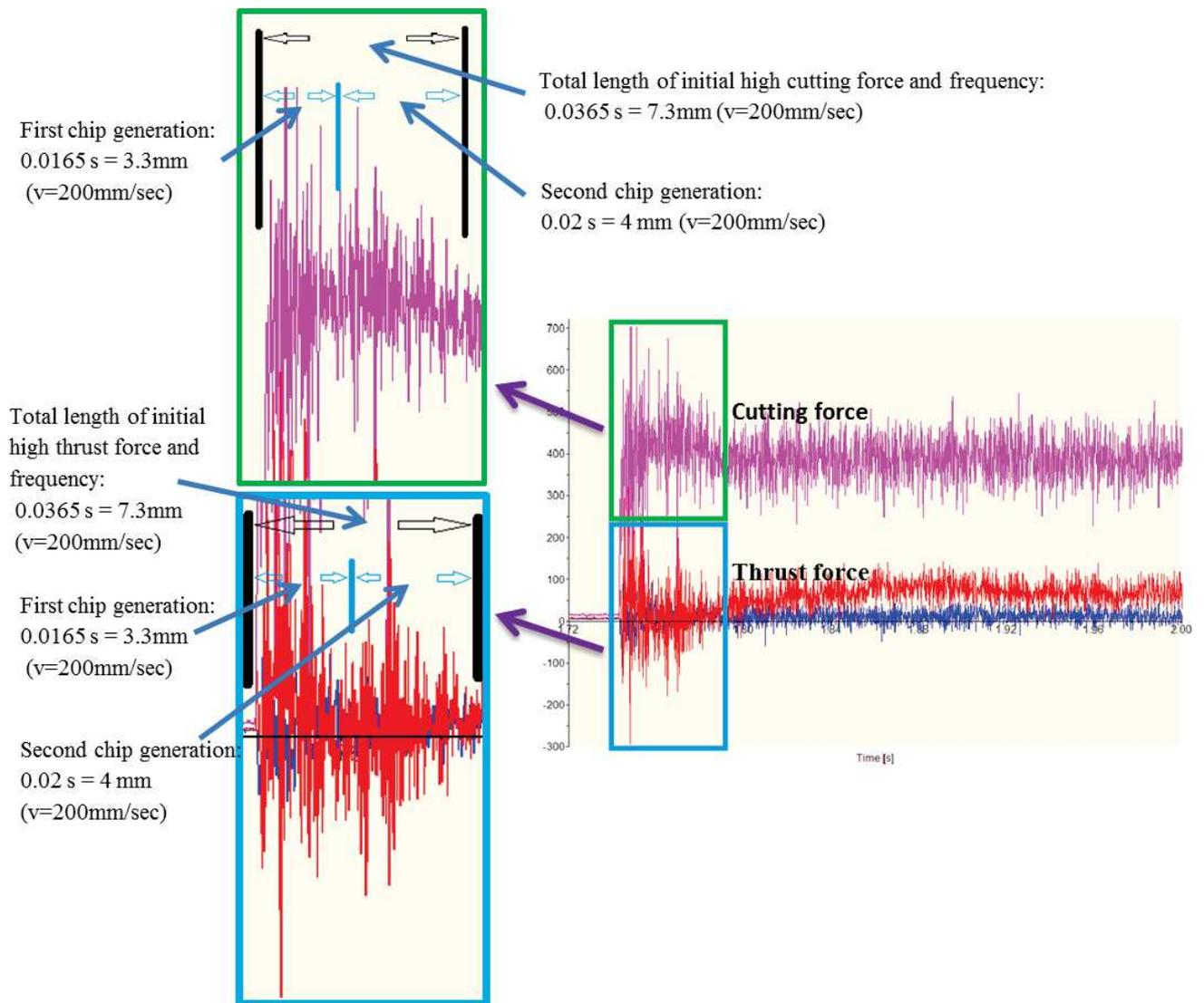
Fig.6. Initial contact forces (experimental).
