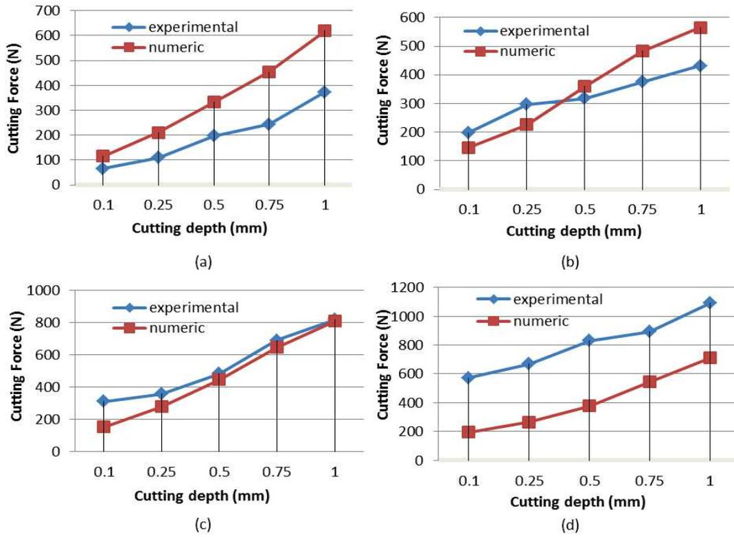
Fig.4. Comparison of numerical and experimental cutting forces: (a)  $0^\circ$  fiber orientation (b)  $45^\circ$  fiber orientation (c)  $90^\circ$  fiber orientation and (d) at  $135^\circ$  fiber orientation.
