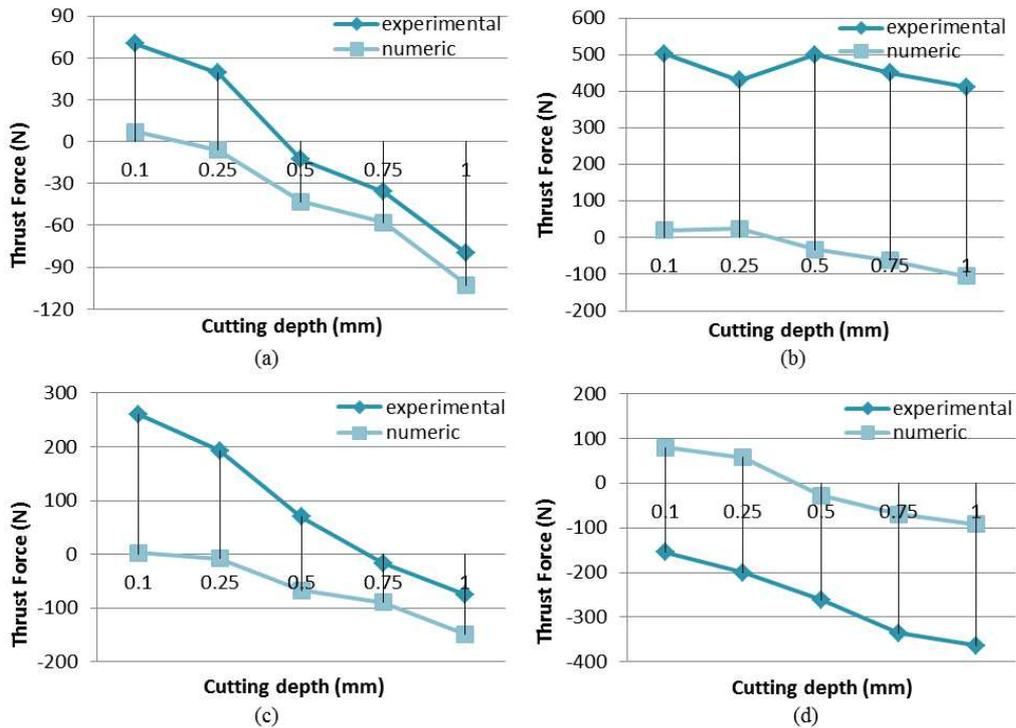
Fig.5. Comparison of numerical and experimental thrust forces: (a)  $0^\circ$  fiber orientation (b)  $45^\circ$  fiber orientation (c)  $90^\circ$  fiber orientation and (d) at  $135^\circ$  fiber orientation.
