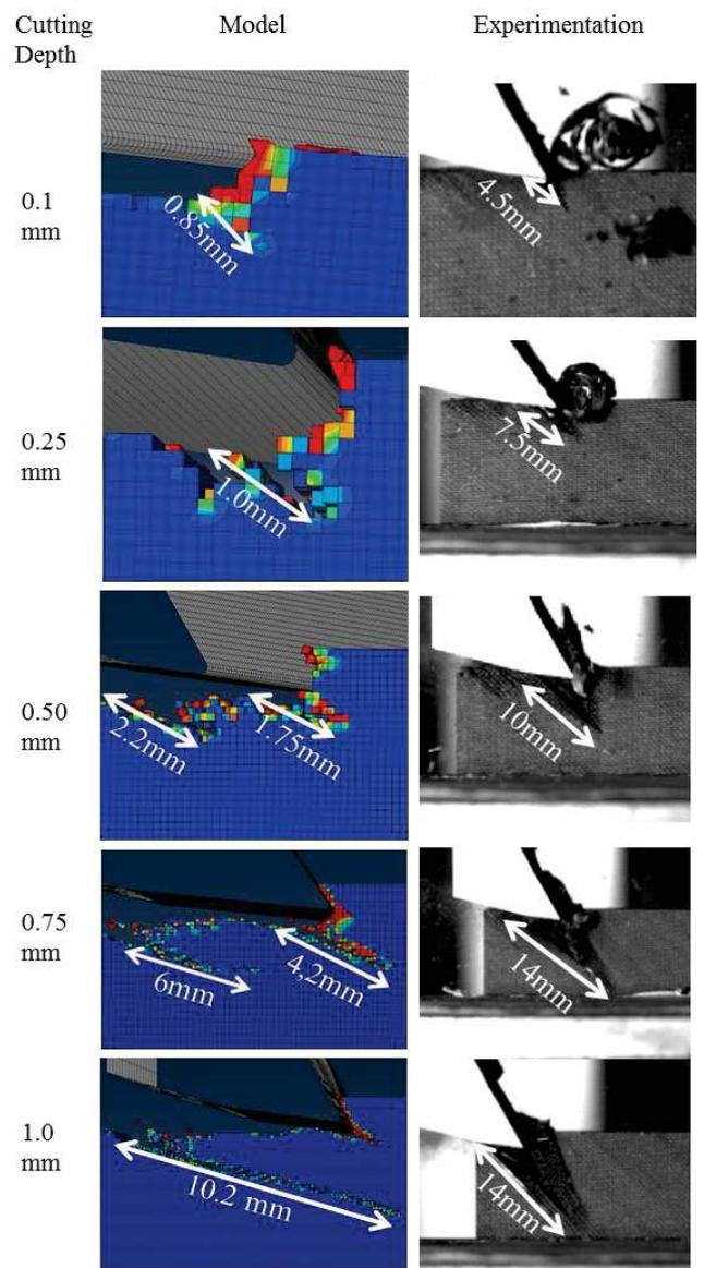
Fig.10. Numerical and experimental fiber-matrix interface crack as a function of cutting depth at 135° fiber position.
