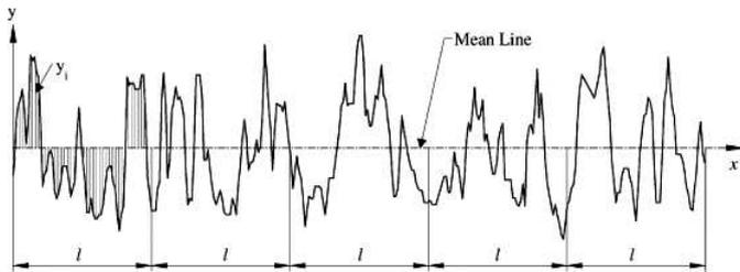
Fig.7. Arithmetic average height,  $R_a$  [Gadelmawla et al., 2002].
