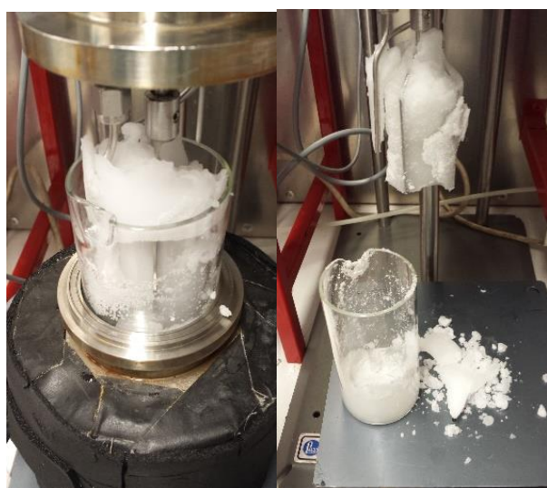
Figure S4. Snapshots of the state of the system after hydrate formation without surfactant.
