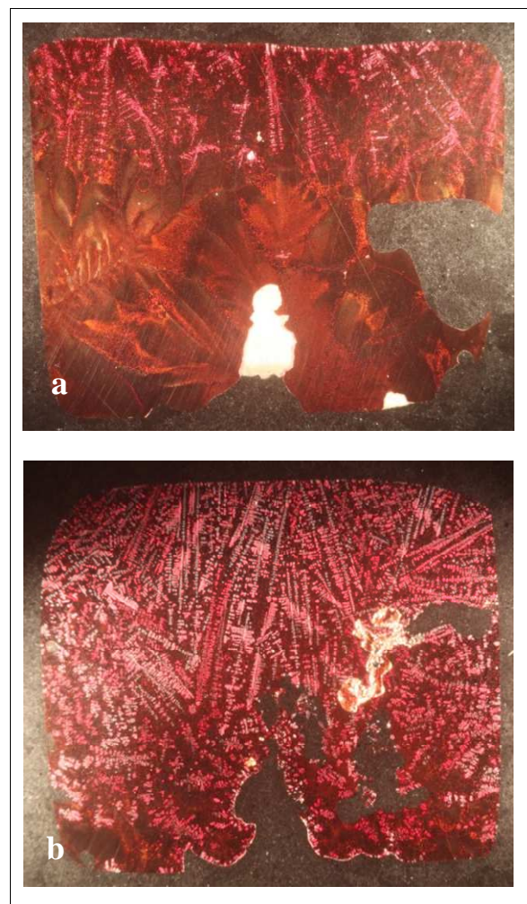
Figure 3: Bright field light microscopy macrographs of the vertical section of samples 1 (a) and 2 (b). The samples were 16 mm in diameter.
