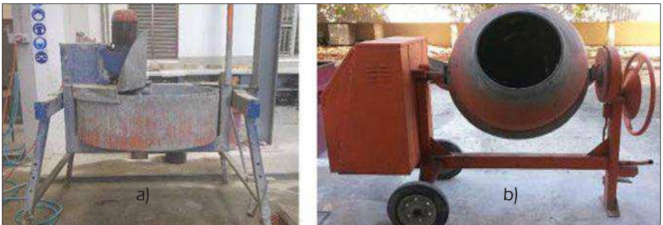
Fig. 6: a) Pan mixer and b) tilting-drum mixer (Lerch, 2018)
