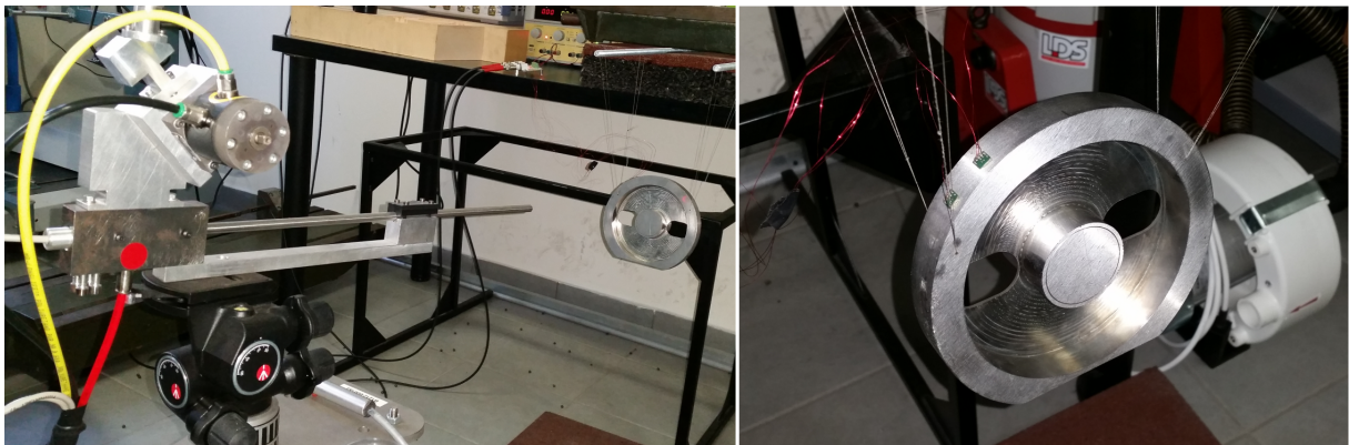
Figure 5: Left: suspended disc, automated pneumatic ball shooter. Right: Xtrinsic accelerometer attached on the side of the rim.
