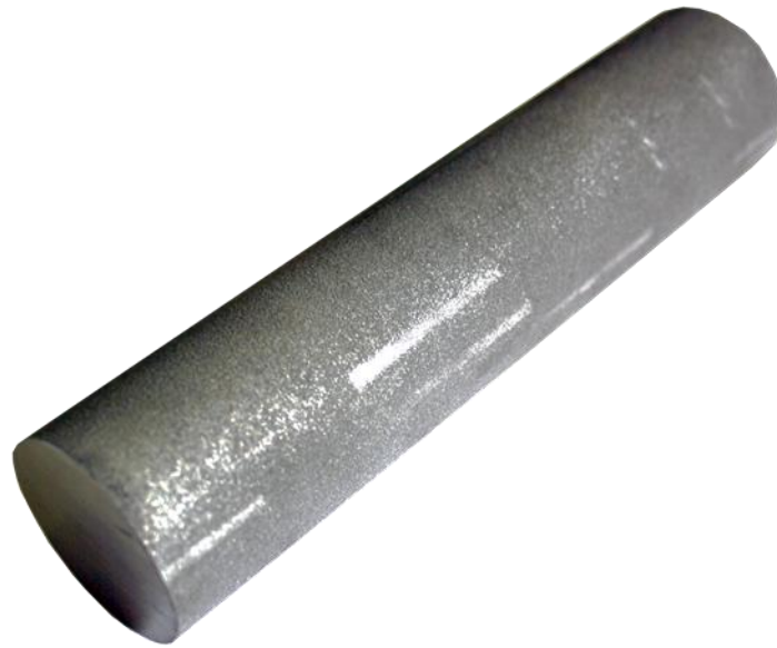
Figure 3.1 As built cylindrical workpiece made of EBM Ti6Al4V.
