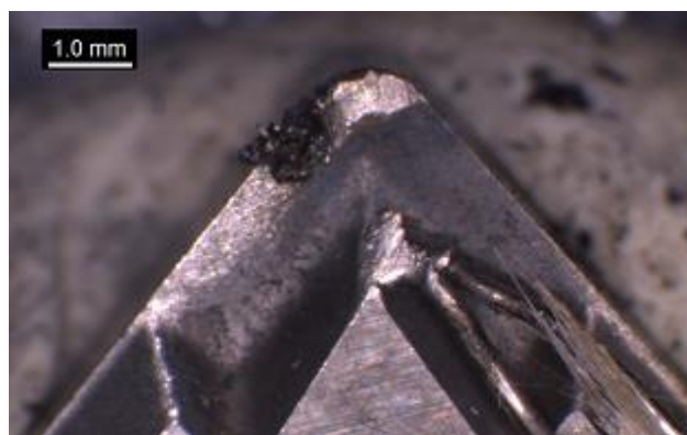
Figure 2.22 K type thermocouple glued on the tool rake face to acquire the cutting temperature during rough turning of Ti6AL4V alloy under dry and cryogenic cooling by Bermingham et al. [32].
