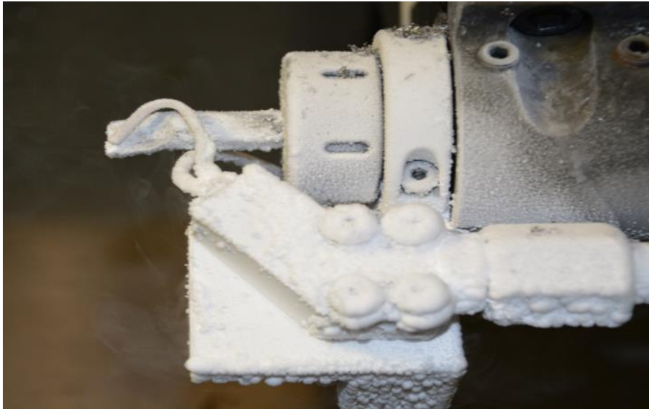
Figure 7.9 Tool holder and nozzles set up completely frozen during cryogenic machining.
