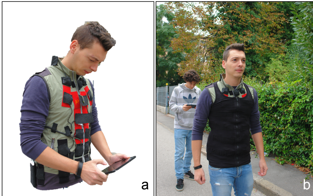
Figure 39. The inner layer of the vest with the actuators placed on the torso (a). An overview of the complete vest with the outer layer on (b)
