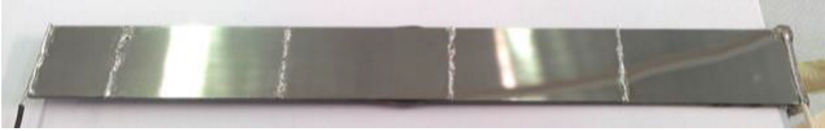
FIGURE 5.35: The final prototype equipped with silicon dummy chips. The tin soldering lines for the electrical interconnection of the Platinum film and the two electrodes at the extremities are also visible.
