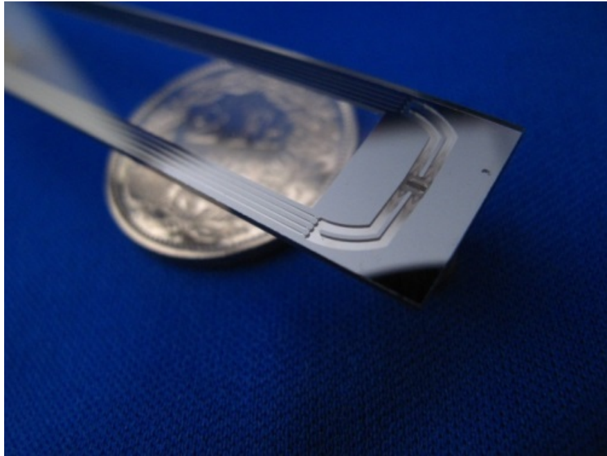
FIGURE 5.3: First prototype of silicon frame with embedded microchannels
