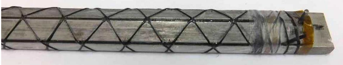
FIGURE 5.53: Mould for the winding process.
