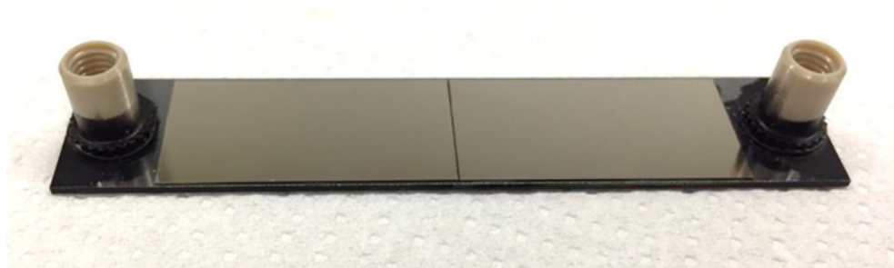
FIGURE 5.7: The silicon frame prototype equipped with Peek connectors and two silicon dummy chips.
