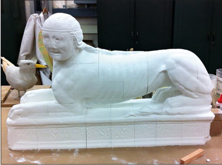
Fig. 6 – The twenty 3D printed areas of the Sphinx joined together during the assembling stage made by the Peabody artist Michael Anderson.
