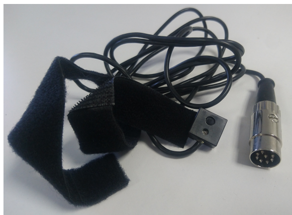
Figure 2.5. The IR Plethysmograph Finger Clip from ADInstruments with a wavelength of 950 nm that has been used for PPG data collection in our biomedical laboratory.
