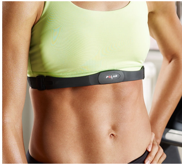
Figure 3.1. An ECG chest belt [18] which can be used to monitor the heart rate during physical activity.
