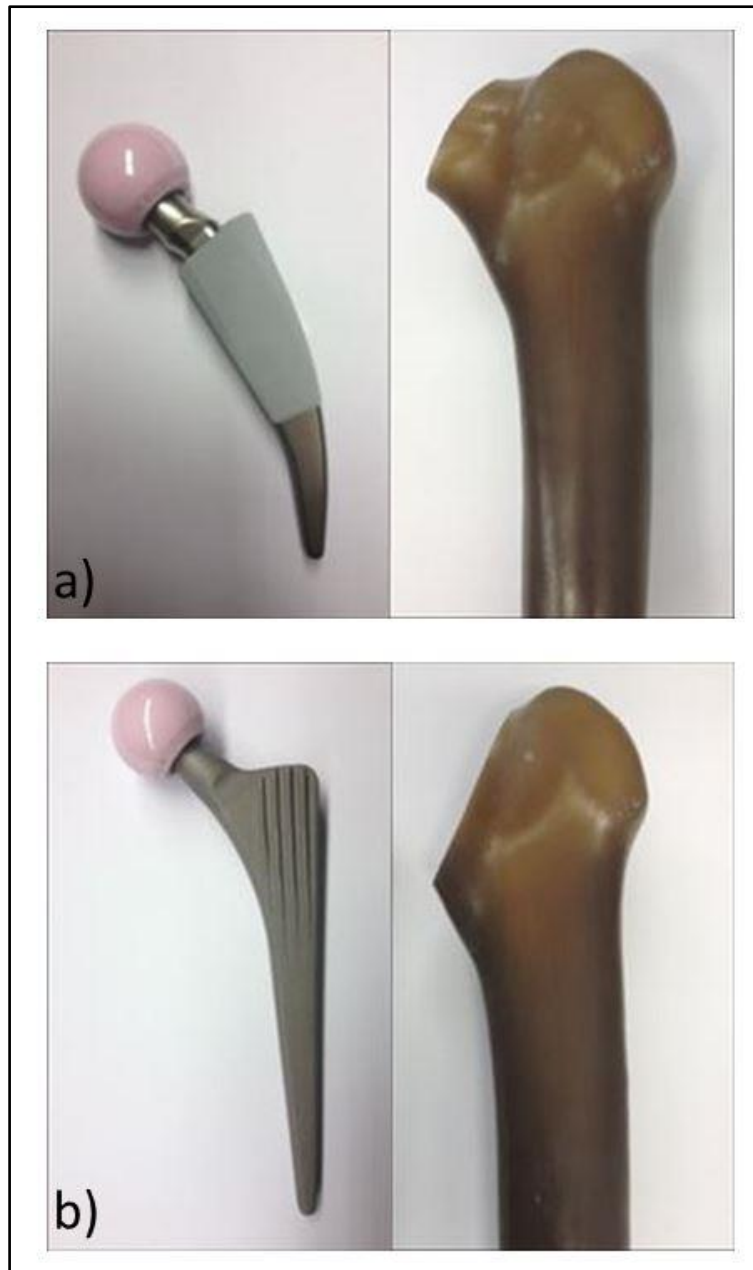
Fig. 21: Sawbones with different femoral head osteotomies according to the stem design:
