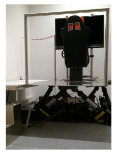
Figure 1.9: 6-degree-of-freedom hexapod motion platform
