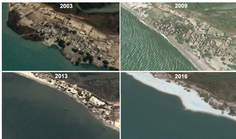
Figure 4. The breach intervention successfully protected the city of Saint Louis, but led to the complete destruction of the village of Doun Baba Dièye. Villagers had to migrate, without compensation for their loss of homes, land, and livelihoods.
