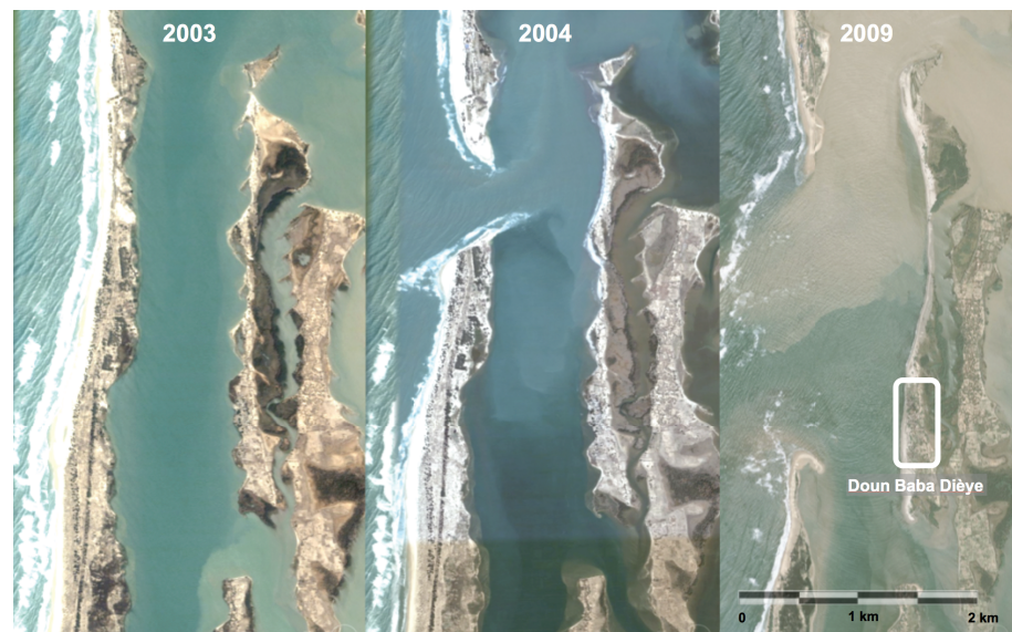
Figure 2. Satellite imagery from Google Earth shows dramatic changes since opening the breach to accelerate drainage of the Senegal River and reduce flood risk in a city further north. The villagers of Doun Baba Dièye were not part of the decision-making process to alter the sand barrier that protected it from the open ocean. Six people were killed in 2010 during what in the eyes of the community was an unprecedented coastal storm.
