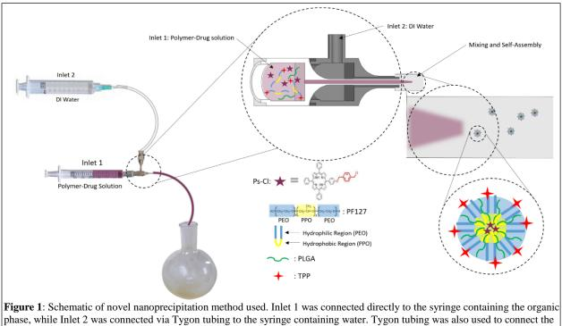
phase, while Inlet 2 was connected via Tygon tubing to the syringe containing water. Tygon tubing was also used to connect the needle to the flask. It was made sure that the end of the tube was underneath the surface of the fluid in the flask. Upon reaching the outlet of the needle, the two phases underwent mixing, and the amphiphilic polymers self assembled trapping the hydrophobic Ps-Cl in their core.
