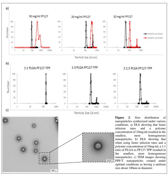
There was less of a chance for the amphiphilic polymer molecules to interact with each other – and less polymer molecules to interact overall – to form larger aggregates. Thus, only small nanoparticles, all approximately the same size, resulted from a polymer concentration of 10mg/ml and infusion rates of 20ml/hr for water and 4ml/hr for oil.
