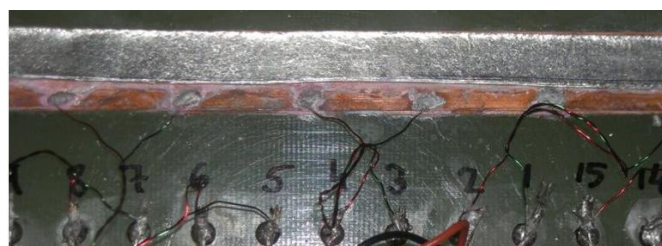
Fig. 3: Sample 2 – Sn foil (8 mm wide, 1 mm thick) position and cable wiring.
