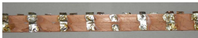
Fig. 4: Sample 3 – soldering pattern. Width of the copper shunts (strips) is 5 mm and thickness 0.1 mm.
