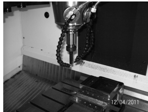
FIGURE 1. Position of MQL nozzles in the high speed milling
