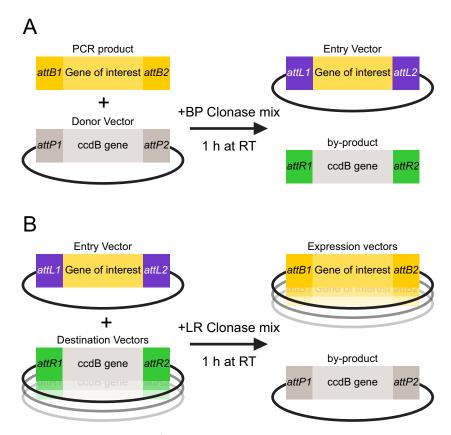
Figure 2.1 | The principle of Gateway<sup>®</sup> cloning. (A) An "Entry Vector" is created through site-specific recombination that is catalysed by a "BP Clonase<sup>™</sup>" enzyme mix as described in the text. (B) The "Entry Vector" is used in a second step to recombine the gene of interest into one of many commercially available "Destination Vectors", yielding Expression vectors in which the protein of interest is usually fused to different affinity-tags.
