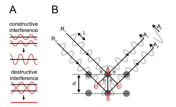
Figure 2.7 | Graphical representation of Bragg's law. (A) Examples of constructive and destructive interference of two waves. (B) If the ray  $R_2$  travels an additional distance that is an integral multiple of  $\lambda$  then constructive interference with ray  $R_1$  occurs. See text for details.
