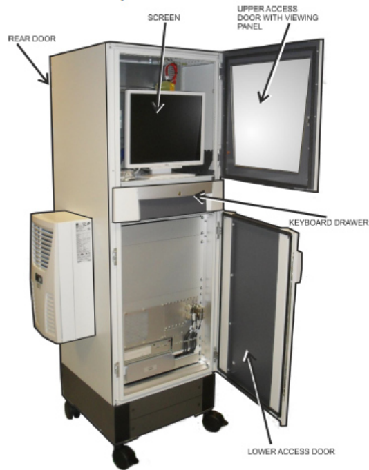
Figure 2. LPF Control Rack Assembly
