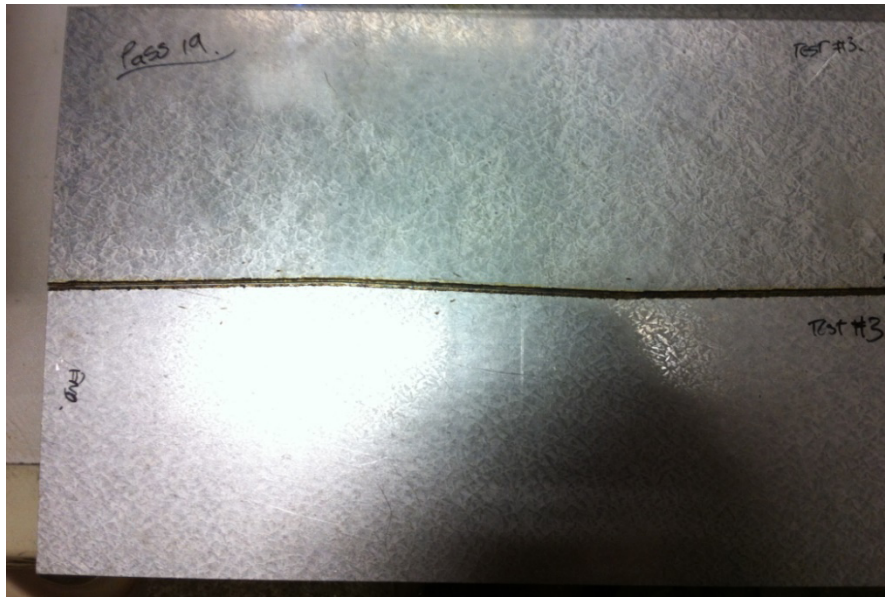
Figure 170 – Physical surface removal trail for the seam tracker.
