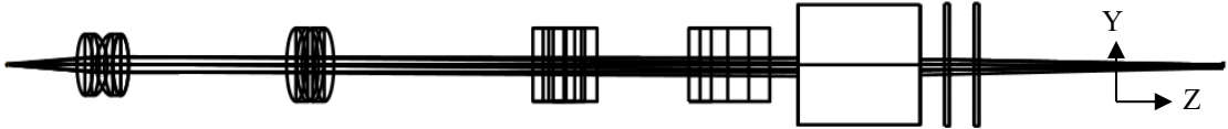
Figure 140 – Architecture 2 YZ plane with Risley and beam steering prism to fit an awkward shape.
