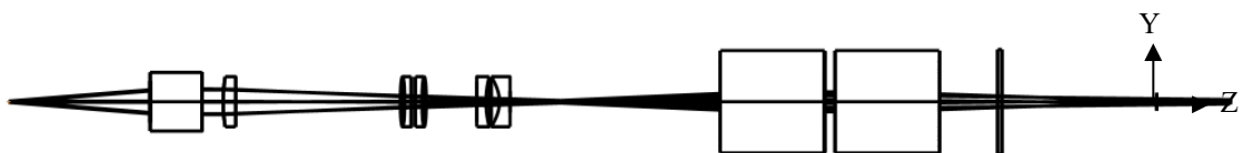
Figure 122 – Architecture 1 XZ plane detailing position of Risley prisms.
