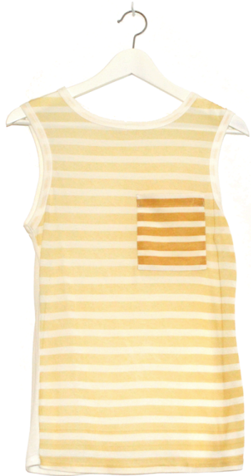
Figure 4.12. A basic sleeveless T-shirt produced using the technique of increasing the number of passes of dye over the fabric during screen-printing.
