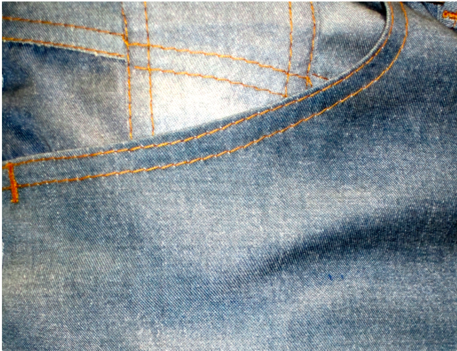
Figure 6.32. A close up of the pocket showing the digital print effect creating a faded, worn look.
