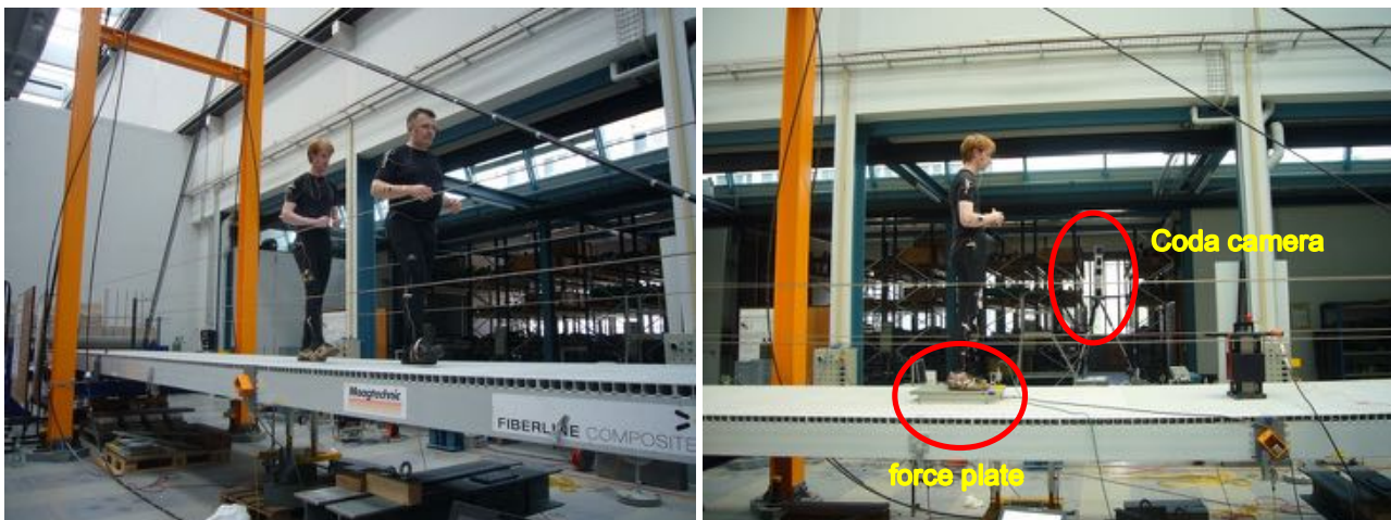
Figure 2 Coda system at EMPA laboratory measuring forces and response due to walking and jumping.
