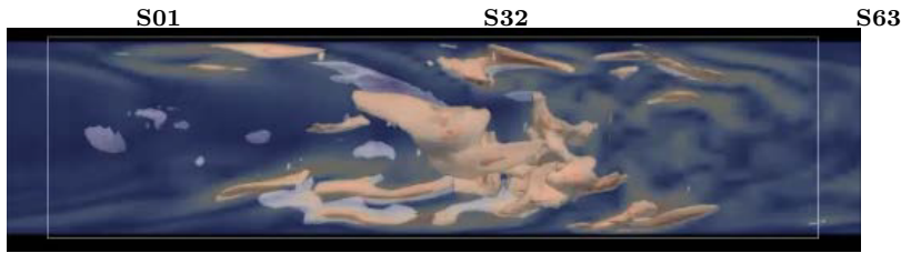
Fig. 1 DNS of a turbulent puff in pipe flow at Re_m = 2250 . Iso-surfaces of the total kinetic turbulent energy e_{tot} = e_{\perp} + e_z plotted in a 4D-length window, centered around the cross-section S32 with e_{\perp}^{(max)} .
