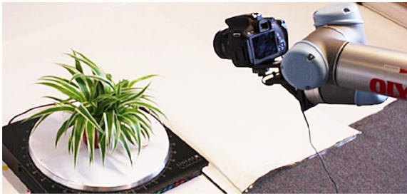
Fig. 2. The Active Vision Cell (AVC) hardware components: the LT360EX high precision turntable (left) and the Canon 650D mounted on the UR5 robot arm
