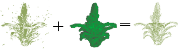
Fig. 6. Model merging. (a) the original point cloud data consisting of outliers, (b) the PPR representation containing unverified voxels, (c) the merged model with the removal of outliers.
