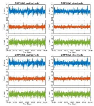
Fig 8 Baseline errors of short-baseline formed by LEICA receiver pair (top) and PANDA pair (bottom) estimated with DD method. In the data processing, we use the empirical model and the refined model respectively as the
