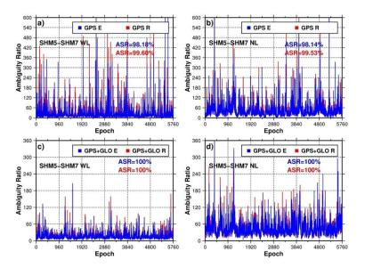
Fig 12 Ratio of single epoch ambiguity resolution of SHM5-SHM7. (GPS E – GPS single system with empirical stochastic model, GPS R – GPS single system with refined stochastic model, G+R R – GPS/GLONASS system with refined stochastic model). The sampling rate of the data has been re-sampled to 15s by TEQC software (Estey and Meertens 1999).
