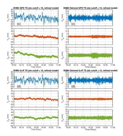
Fig 17 Structural displacements and their high frequency components for refined model schemes (c) and (d).
