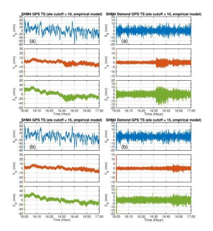
Fig 15 Structural displacements and their high frequency components for empirical model schemes (a) and (b).
