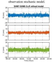
Fig 9 Baseline errors of integrated GPS and GLONASS data processing for SHM7-SHM5 with refined stochastic model.
