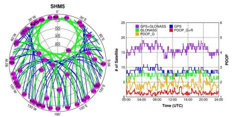
Fig 2 Sky plot and the number of visible satellites with PDOP time series for the whole day. (In the right panel, G – GPS only; G+R - GPS+GLONASS)
