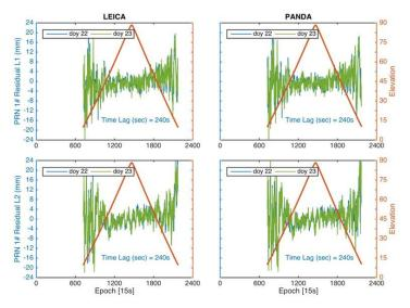
Fig 6 Residual and elevation time series of PRN 1# in two consecutive days. The residual time series of day of year 23 was moved backward for 240 seconds (16 epochs for 15s sampling rate).
