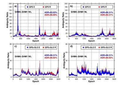
Fig 20 Ratio of single epoch ambiguity resolution of SHM4-SHM1. (GPS E – GPS single system with empirical stochastic model, GPS R – GPS single system with refined stochastic model, G+R R – GPS/GLONASS system with refined stochastic model). The sampling rate of the data has been re-sampled to 1s by TEQC software (Estey and Meertens 1999).
