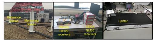
Fig 1 Zero and short baseline experiment setup, the receivers and the splitter.
