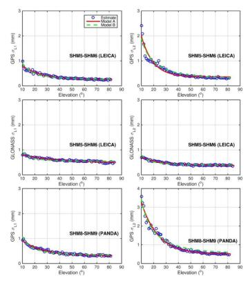
Fig 4 Estimated elevation-dependent precisions and their modeling with the two predefined models. As proposed by Li et al. (2015a, 2016), the predefined functions of elevations, exponent type and sine type, can achieve a good result in descripting the observation precisions with elevation changes. Then, we employ the following two models to fit the precisions:
