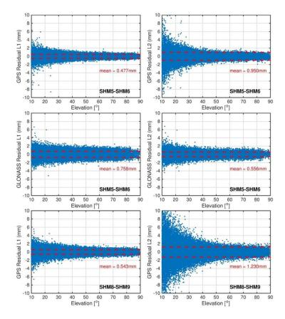
Fig 3 Residual time series of all satellites changes with elevation variation from 10° to 90°. The red dash line is the mean precision of all satellite observation.
