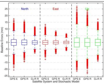
Fig 10 Box plots of SHM7-SHM5 baseline errors. (GPS E – GPS single system with empirical stochastic model, GPS R – GPS single system with refined stochastic model, G+R R – GPS/GLONASS system with refined stochastic model)
