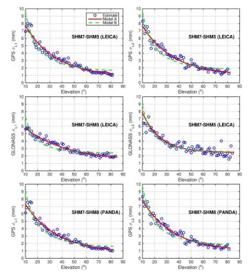
Fig 7 Estimated elevation-dependent precisions and their modelling with two predefined models in short-baselines.
