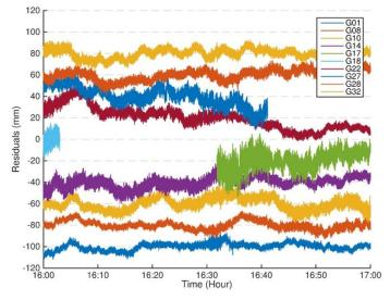
Fig 16 Posteriori residuals for GPS L1 observations. There is an upward shift of 20 mm successively from G01.
