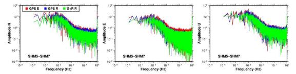
Fig 11 Spectral analysis for the data processing of SHM5-SHM7. (GPS E – GPS single system with empirical stochastic model, GPS R – GPS single system with refined stochastic model, G+R R – GPS/GLONASS system with refined stochastic model).
