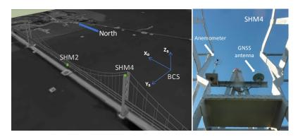
Fig 13 The defined Bridge Coordinate System (BCS) and antenna setting-up at SHM4.
