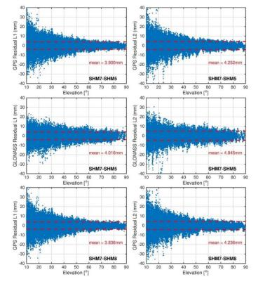
Fig 5 Residual time series changes with the elevation for all satellites. The red dash line is the mean precision of all residuals.
