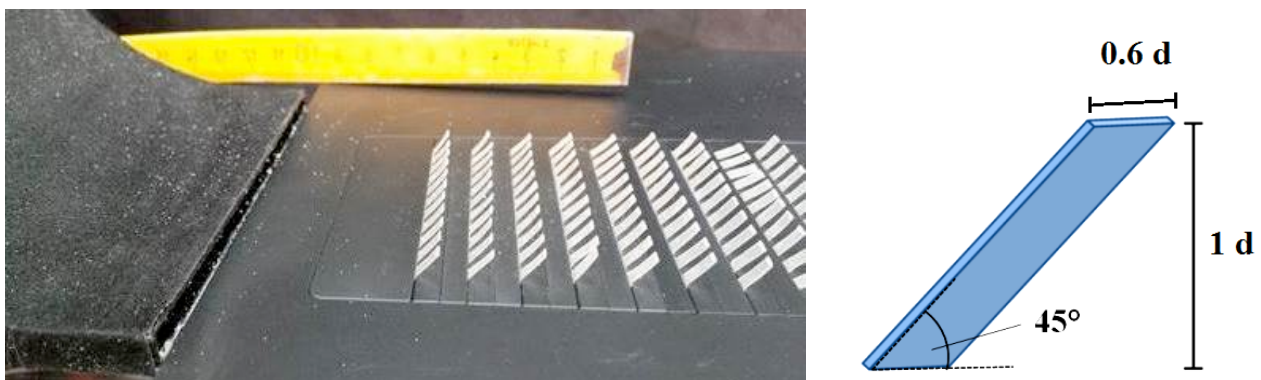
Fig. 2 Used flap array with transparent foil flaps of a height of 1 d and a width of 0.6 d with a spanwise pitch of 0.6 d and a streamwise interspacing of 2 d . The first row is positioned at 8 d downstream of the nozzle exit. As illustrated in the right sketch, the flaps are elevated from the wall with a deployment angle of 45^\circ
