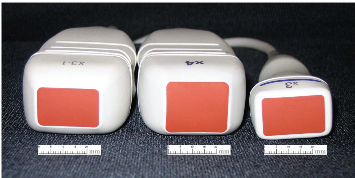
Figure 2 Size of the different 2D and 3D Philips transducers, from left to right: 3D-X3-1 (24 x 15 mm), 3D-X4 (24 x 20 mm) and 2D-S3 (24 x 15 mm).
