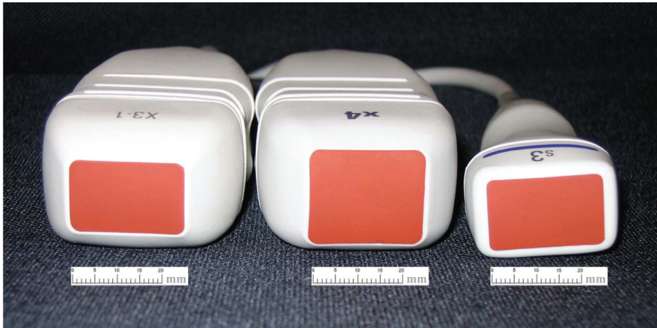
Figure 6 Size of the different Philips transducers, from left to right: 3D-X3-1 (24 x 15 mm), 3D-X4 (24 x 20 mm) and 2D-S3 (24 x 15 mm).
