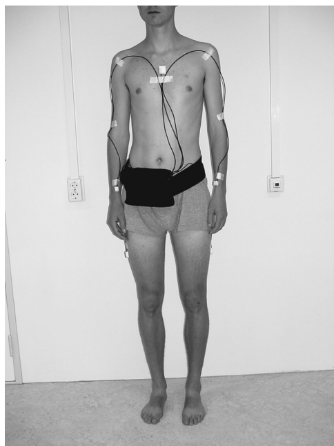
Figure 1. A subject wearing the Upper Limb Activity Monitor, with accelerometers on the forearms, trunk, and thigh(s) and the data recorder in a waist-worn machine-washable bag.
