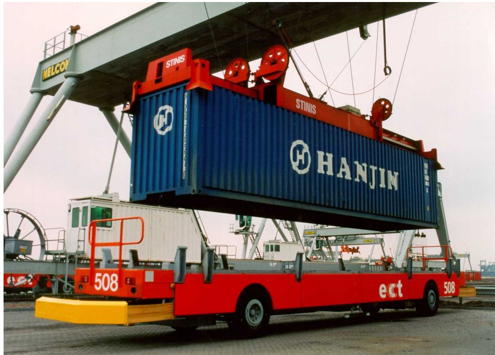
Figure 3.3: Loading of an AGV by an ASC (photo: courtesy of ECT)
