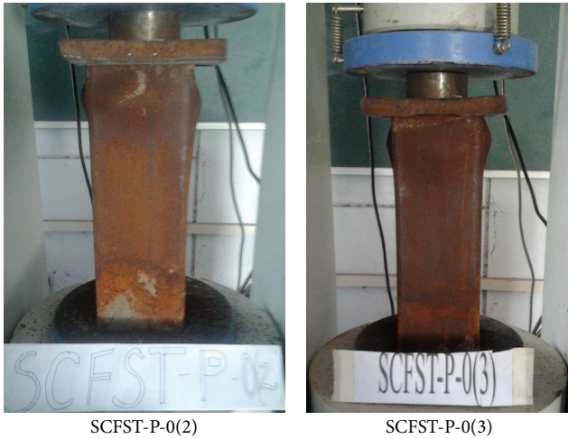
FIGURE 4: Failure pattern of square CFST column subjected to partial/local compression.
