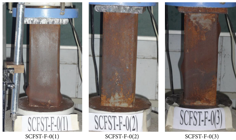
FIGURE 3: Failure pattern of square CFST column subjected to full compression.
