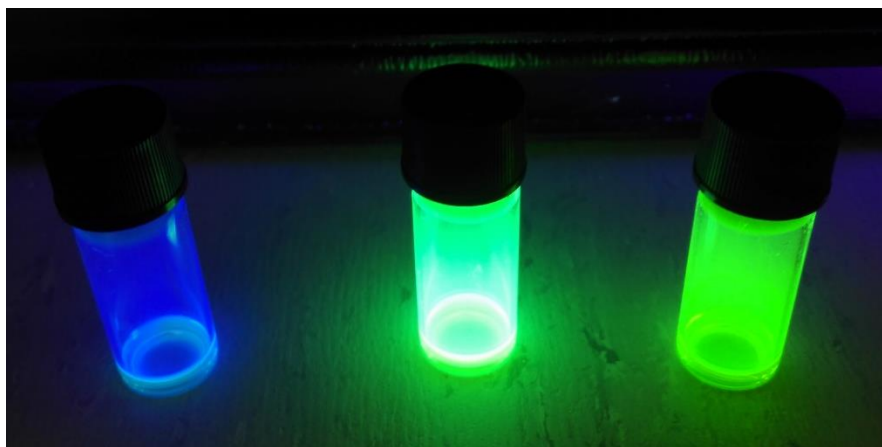
Figure 19 – 2 month old nanocrystal solutions of \text{CsPbBr}_{1.5}\text{Cl}_{1.5} (left) \text{CsPbBr}_3 (centre), and \text{CsPbBr}_{1.5}\text{I}_{1.5} (right). Note that the \text{CsPbBr}_{1.5}\text{I}_{1.5} solution appears green rather than yellow, indicating that the solution has degraded.
