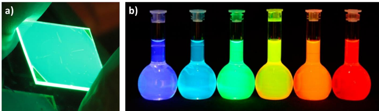
Figure 31 - A highly luminescent film of n=3 layered perovskite. b) Solutions of \text{CsPbX}_3 perovskite nanocrystals (Image source [74]).
