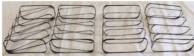
Figure 2-25: CFRP spiral shear reinforcement (Image courtesy: Grant (2013))
