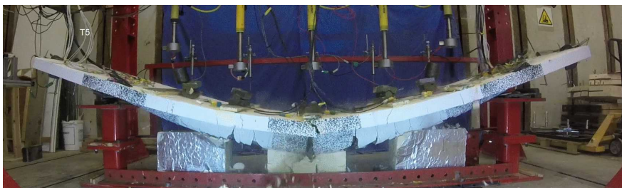
Figure 6-26: Flexural failure in T5
