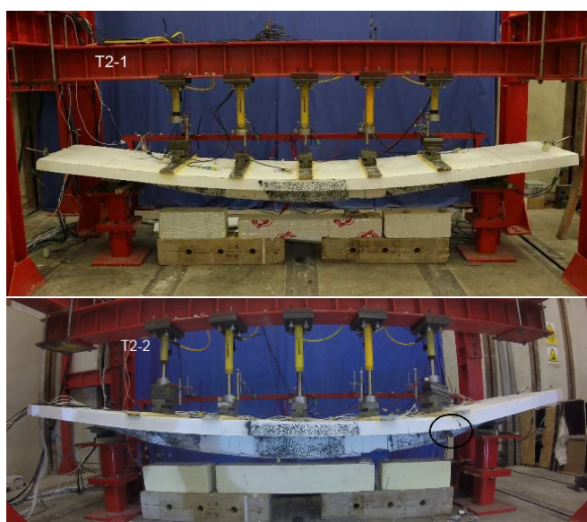
Figure 6-30: End slip failure in T2-1 and T2-2
