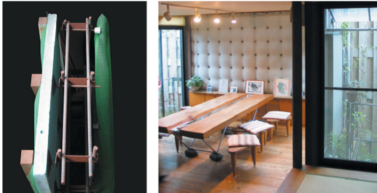
Figure 2-4: Zero waste fabric formwork (left) and fabric formed wall (Image courtesy: Kostova (2016))
