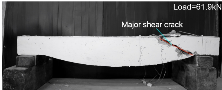
Figure 5-11: Diagonal tension failure of TP2-1
