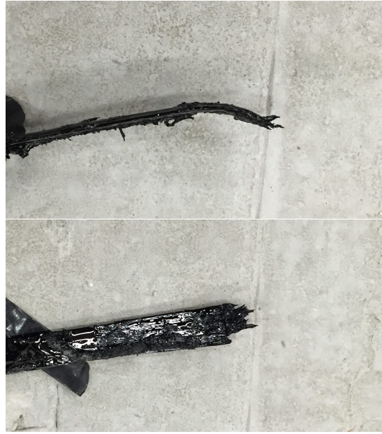
Figure 4-10: Failure of W-FRP shear links: WB_I (top) and WB_II (bottom)
