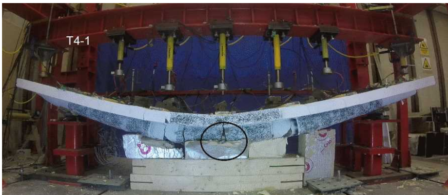
Figure 6-25: Flexural failure in T4-1
