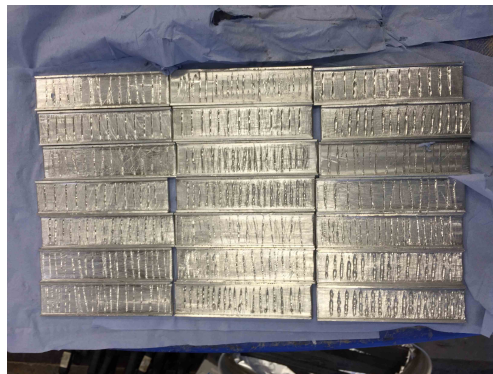
Figure 4-4: Notched aluminum anchor tabs
