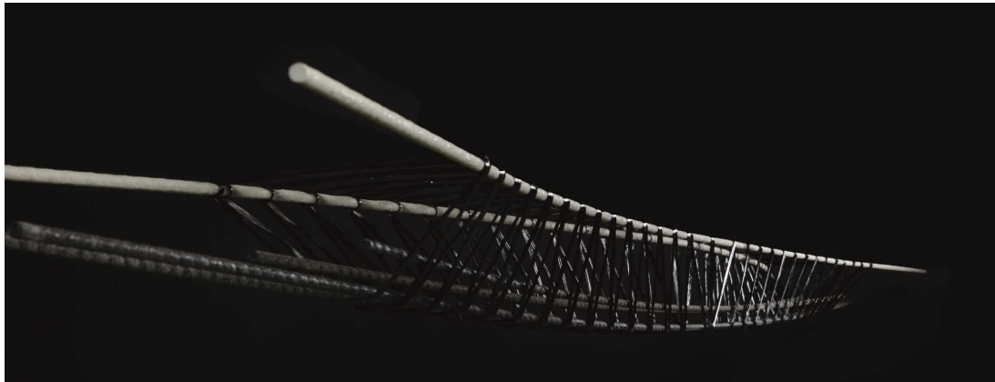
Figure 1-4: Wound FRP cage for concrete beam (Image courtesy: John Orr)
