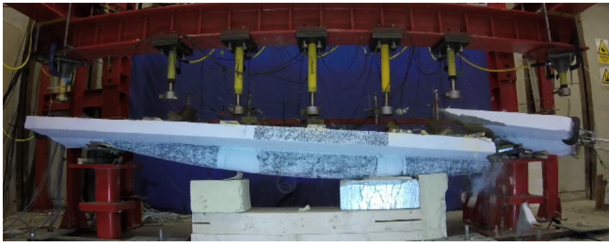
Figure 6-21: Shear failure in T1
