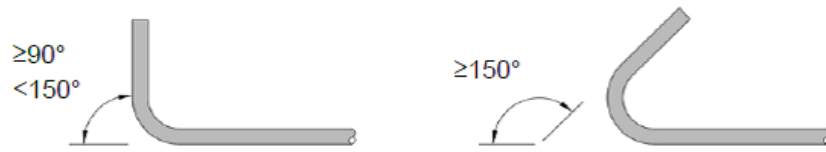
Figure 2-31: Traditional bends and hooks at anchorage zone
