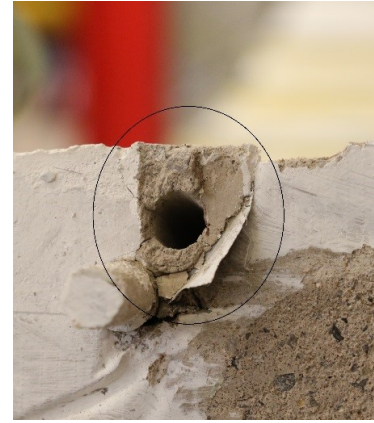
(b) End slip of longitudinal bar
