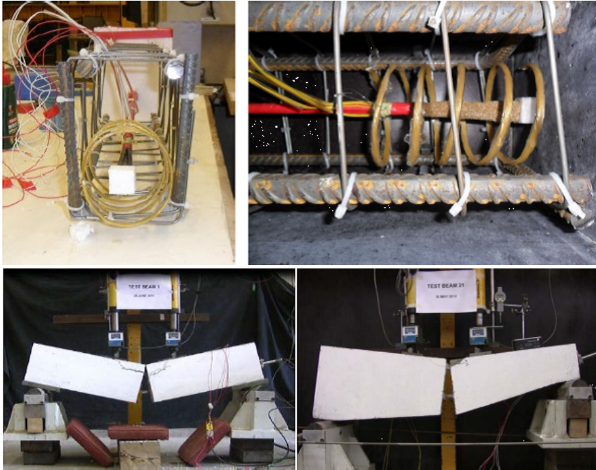
Figure 2-33: Pull-out tests of 'splayed anchorage's (Image courtesy: Kostova (2016))
