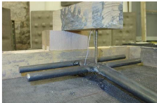
Figure 2-29: ‘T bar’ anchorage (Image courtesy: Lee (2011))
