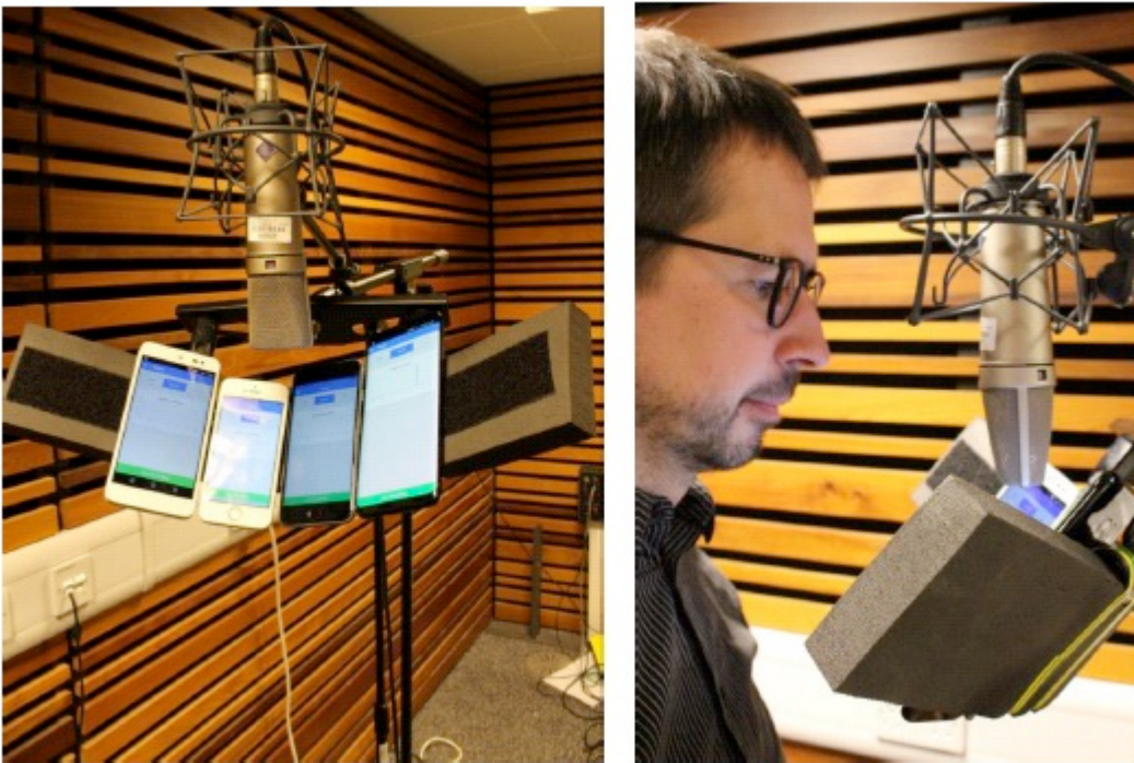
Figure 1- The experimental setup with an array of four smartphone devices and reference microphone.
