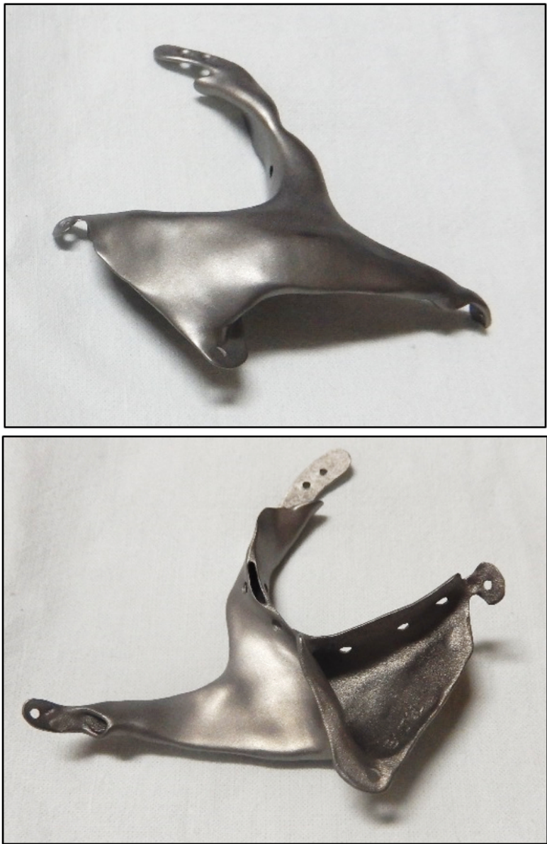
Figure 9. Implant fabricated from Titanium alloy
