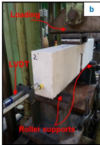
Figure 3. Hinged beam test set-up: (a) front view and (b) side view
