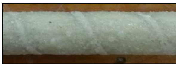
156 157 158 (a) Helically wrapped with sand coated surface (type A) 159
