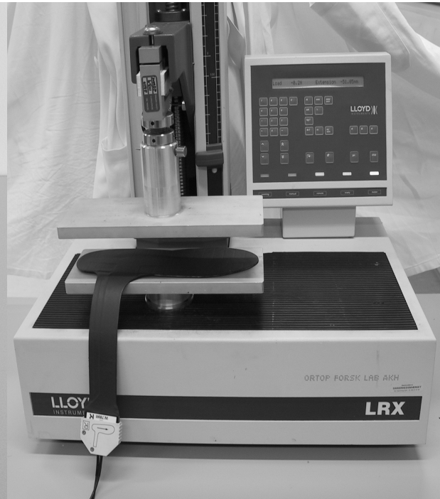
Figure 2. The dynamic loading device (Lloyd instruments Ltd, Hampshire, UK) with a Pedar insole placed between two steel plates.
