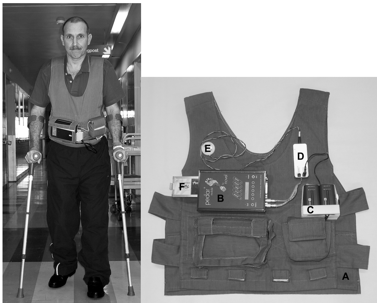
Figure 1. The Pedar system with a custom-made battery unit placed in a custom-made vest (right) worn by a patient (left). The accelerometer is connected to the Pedar system and fixed on the middle front part of the contralateral thigh. (a = custom made vest; b = Pedar box; c = battery unit; d = electronic device; e = accelerometer; f = 40 Mb flash card)
