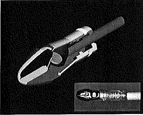
Figure 6. View on the design of the catheter tip combining spark erosion and ultrasound imaging and the fabricated tip of the catheter prototype as applied in the experiments. Both the active electrode, surrounded by ceramics, and the circular ultrasound transducer can be observed. In the photograph the sleeve covering the ultrasound transducer is withdrawn to allow fluid filling of the cavity.
