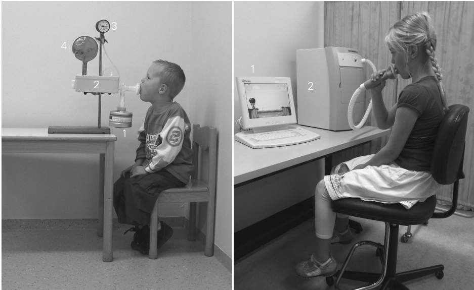
Figure 1.3. Measurement of nitric oxide fraction in exhaled air at 4 and 8 years (a). Offline measurement in a 4-yr-old boy. 1: NO scrubber, 2: dynamic flow restrictor (50 mL/s), 3: manometer, 4: mylar balloon. (b). Online measurement of the nitric oxide fraction in exhaled air in an 8-yr-old girl. 1: computer animation gives visual feedback to maintain constant expiratory flow (50 mL/s), 2: online nitric oxide analyzer with built-in NO scrubber and dynamic flow restrictor.
