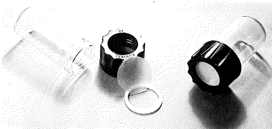
Fig. 4-16. Glass-vial for controlled freezing of aortic valves, constructed of pyrex glass, and a screw-cap of bakelite, with a silicone centre part to form a pressure-valve, necessary whenever liquid nitrogen has entered the vial. A teflon ring is used to assure good closure.
