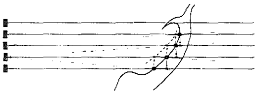
FIGURE 10. Schematic drawing of the left ventricular posterior wall. Targets from the endocardium are distorted in the vertical direction. This effect is more pronounced when the inclination of the target to the ultrasonic beam increases until at a certain angle, there is no more echographic return. This results in poor visualization of the apex. The internal shape of the left ventricle is distorted because the true endocardial surface (solid line) is erroneously displayed by the dotted line.
