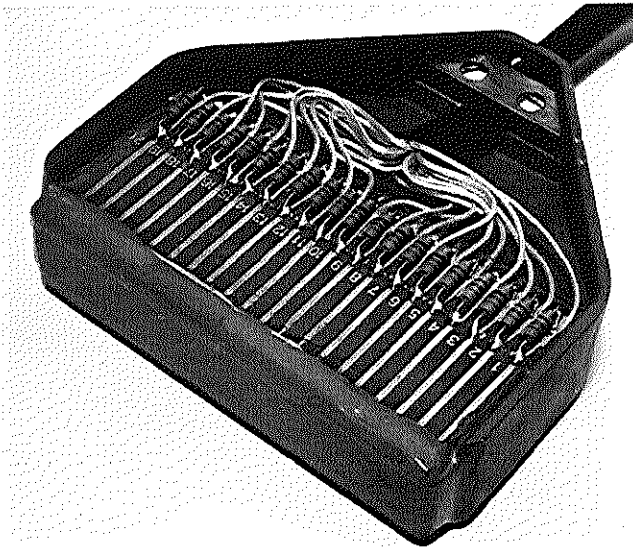
Figure 1. Multiscan transducer. It contains 20 elements and the active surface has a width of 1 cm and a length of 8 cm.
