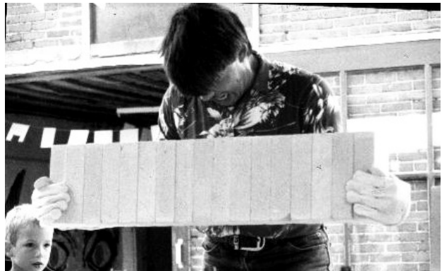
Figure 4. Illustration of principle of form and force closure: the combination of surfaces with a specific friction coefficient and compressive force provides stability.
