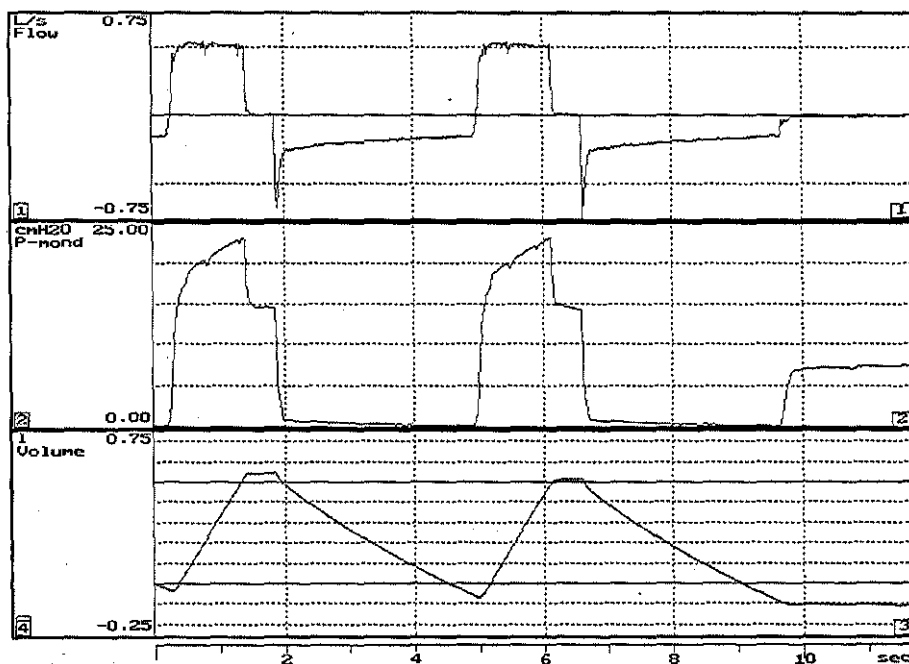
Figure 5. Measurement of static iPEEP. By occlusion of the airway at end-expiration a plateau in pressure is observed, which represents the total PEEP.
